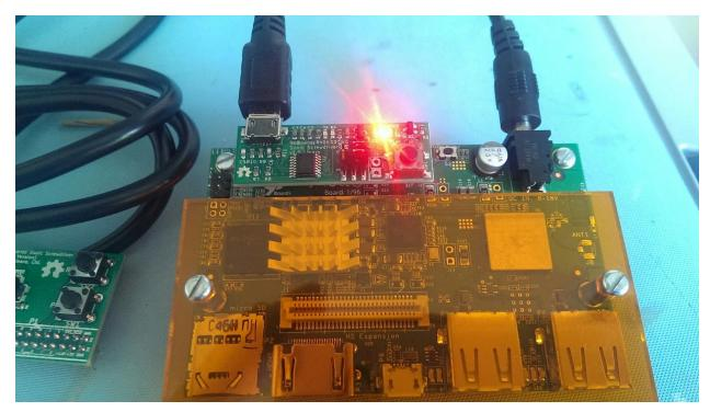
Connect a micro USB cable between P1 and a computer.
