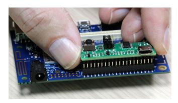
Attach the UART adapter's large 40-pin header (J2) to the LS expansion connector on a 96Boards base board. The connector is oriented with pin 1 beside the USB connector, and pin 40 next to the reset button. DO NOT INSTALL BACKWARDS. The board should be oriented so that the Micro USB connector is facing away from the center of the base board and the edge of the adapter is flush with the baseboard edge.
